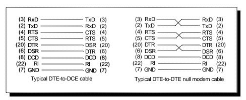
Figure 17 --- Cabling requirements for RS-232-C devices (cables using 25-pin connectors shown)
